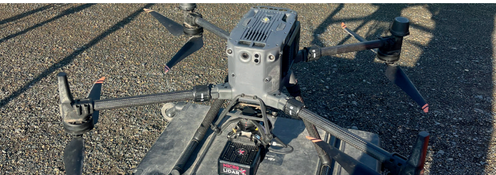
Drone M350 RTK + sensor Micro Lidar
